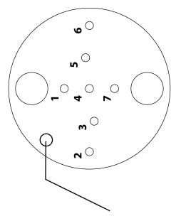
STUD ON MODELS SO EQUIPPED: 12v+ TURN SIGNAL
