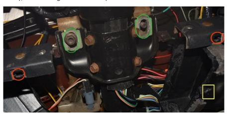
Remove the 3 upper screws . Twist counter-clockwise on the cigar lighter bezel to unscrew.
