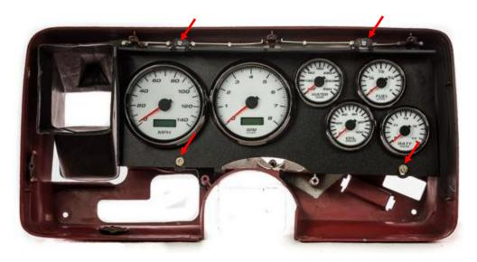
Right side filler panel. Clean side of blackout panel with alcohol. Remove 3M tape and apply piece as shown. If you need to trim it shorter you can with scissors or shears. Test fit before finalizing installation.
