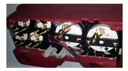
Install in panel. Secure upper tabs (arrows) with original screws. Use supplied #8 hex nuts, washers and lock washers on lower studs (arrows)
