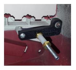
Right side detail. Shows bracket installed. Use a #6x5/8 or a #8x5/8 if the hole is damaged.
