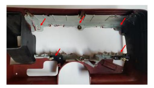
The dash does not require this much trimming but the path shown is the easiest route. Back of cluster will look like this when completed:
