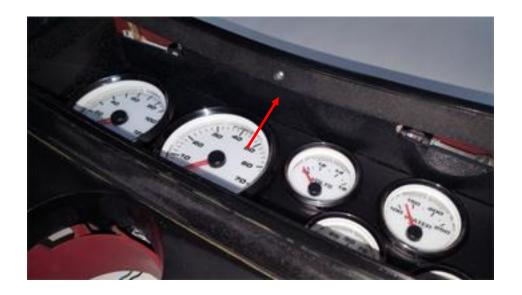
Installation of the cover bezel is reverse of removal. Use the stock screws to re- attach. If needed, top screws are #6x5/8 sheet metal. Install any switches, etc. at this time. After wiring, re-install cluster/bezel/housing assembly back in place.
