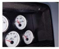
Install cover bezel over cluster. Tuck the lip of the top block out up into the space between the bezel and housing (arrow), this will give a clean look when viewed from the front.
