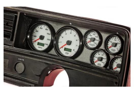
Remove light switch knob and any other protruding switches that may interfere with installation of the bezel. Remove the 10 screws securing the dash bezel and retain for re-use later.
