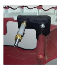
Left side detail. Shows bracket installed. Use a #6x5/8 or a #8x5/8 if the hole is damaged.
