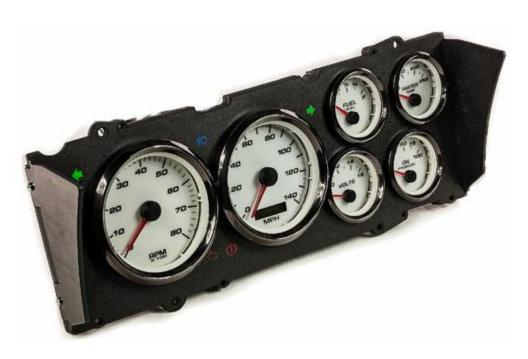
Remove the 4 screws that hold on the front bezel assembly. (under the dash brow). Remove the front bezel. Retain screws for use in re-installation of bezel. The black spacer/blockout plate on the back of the bezel may be used if oyu like. Its not required but you may like the look of leaving it installed..
