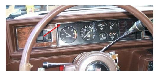
Remove the 4 screws that hold the cluster to the dash. Pull out carefully, reach behind and remove harness and speedometer cable.
