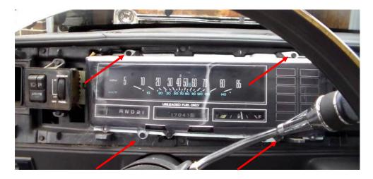
Using a dremel or similar cutoff tool, remove the back "plate" of the dash. This will allow for clearance for the gauges and new wiring. You may need to replace the speedo cable to use on mechanical speedometers. NVU mechanical speedometers use a 5/8-18 thread cable with .104x.104" drive tang. (aftermarket standard)
