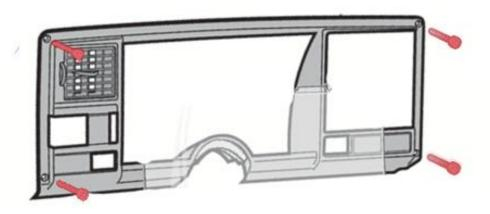
STEP 3: Remove the fasteners securing the OE gauges into the dash, pull gauges cluster assembly from the dash making sure to disconnect the wiring harness connector on the backside of cluster and set to the side for disassembly.
