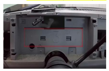
STEP 6: Remove fasteners attaching the Factory Lens and retain factory spacer that is sandwiched between the OE gauges and the lens. *Remove Factory shift Indicator from OE cluster.*
