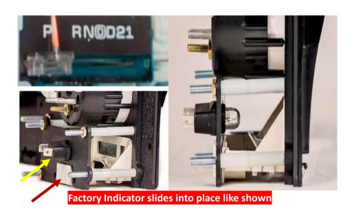
STEP 8: Place your NVU gauges into their desired location in the Direct fit Bracket place gauges thru panel using the 6 included back clamps & hardware to hold the gauges into position.
