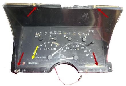
You should be left with just the Spacer piece and factory transmission shift indicator that will be installed to the NVU direct fit bracket later in the install.
