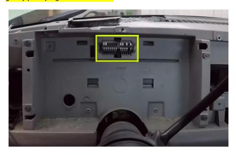
STEP 5: Now that the plastic harness bulge has been removed you should have enough room to slide your NVU Direct Fit Gauge Bracket into place. If the gauges needs more depth, trim red area Outlined below. Caution: Main harness just above steering column
