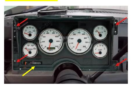
STEP 12: Reinstall factory bezel using 4 factory fasteners
