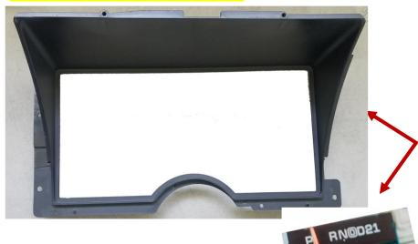
STEP 6.2: Using a rotary tool or other cutting tool to remove the inner portion of the OE gauge spacer. Use care when trimming this plastic piece out, as this factory spacer part is necessary to fill the gaps for a factory look fit.
