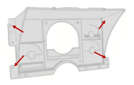
STEP 4: Using a rotary tool or other cutting tool to remove the bulge holding the OE wiring harness connector. *Use care when trimming this plastic piece out, as the harness runs behind the dash at this point.* Splice the wires needed on the harness and gently push plug back into recess
