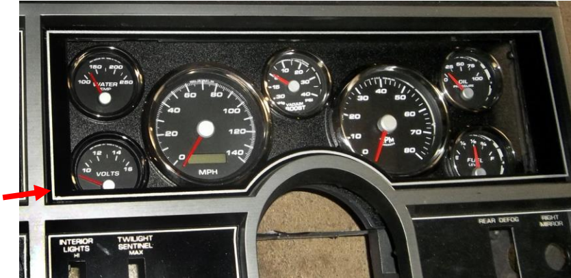
FIG 1. TRIM MASK INSTALLED (ARROW)
