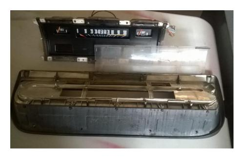
Using a dremel or similar cutoff tool, remove the center panel of the dash. This will allow for clearance for the gauges and new wiring. (aftermarket standard) (The front panel will cover minor flaws.) Cut just inside the lip.
