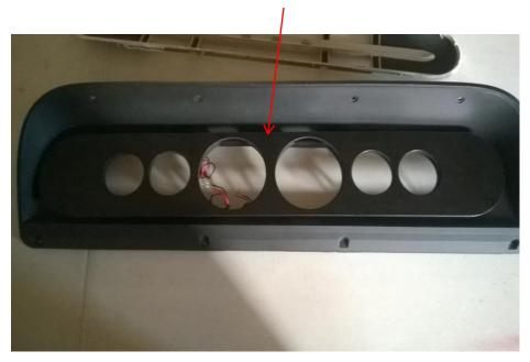
Insert the panel from the front, check that the hi beam is at the top so that the icons are right-side up.
