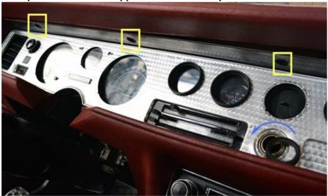
Remove the 6 screws that hold in the 2 piece gauge clusters. Pull out the gauges, remove the wiring plugs, speedometer cable, etc.
