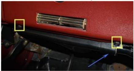
Remove the screw for the air duct (yellow) and drop the duct.
