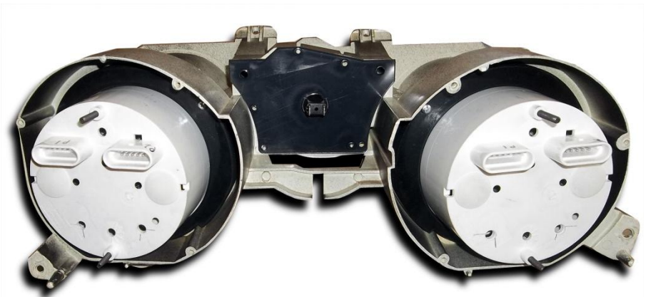
FIG 2 GAUGES INSTALLED FROM REAR, CENTER FILLER LAMP INSTALLED.
