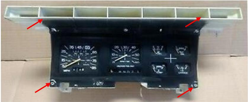
Remove the shift indicator, cable and associated parts.
