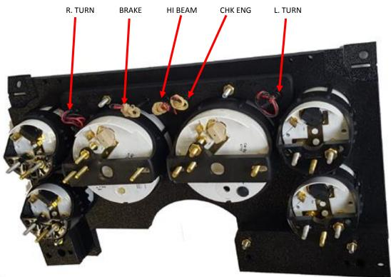
Indicators are LEDs, pre-wired for 12V operation. Red is power black is ground
